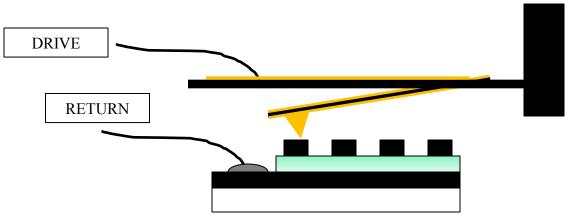
Recent research has demonstrated that electromotive forces act on the conductive cantilever to cause the cantilever to bend during electrical actuation of the capacitor through the cantilever, sending a false displacement signal to the AFM.
