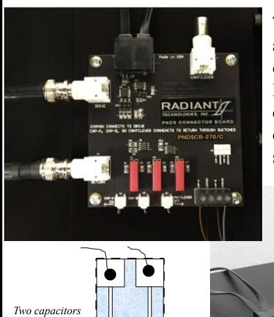
on single substrate. The PNDS has a two channel mux to allow selection of two separate samples on the same substrate on the chuck. The PNDS Sample Selection Board is controlled automatically by Vision but can be operated manually using toggle switches.
